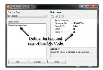
The ability to create and add QR codes, Datamatrix codes and Barcodes has been implemented. The code is initially created as a Custom aperture so that the code can be exported to Gerber and DXF/DWG files.
