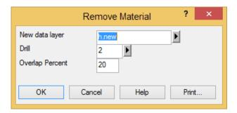
By default the created path is placed on a new Hole/Rout layer and uses the tool number selected from the existing tool table.
