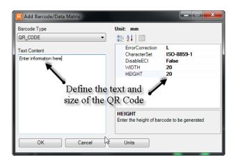
The ability to create and add QR codes, Datamatrix codes and Barcodes has been implemented. The code is initially created as a Custom aperture so that the code can be exported to Gerber and DXF/DWG files.
