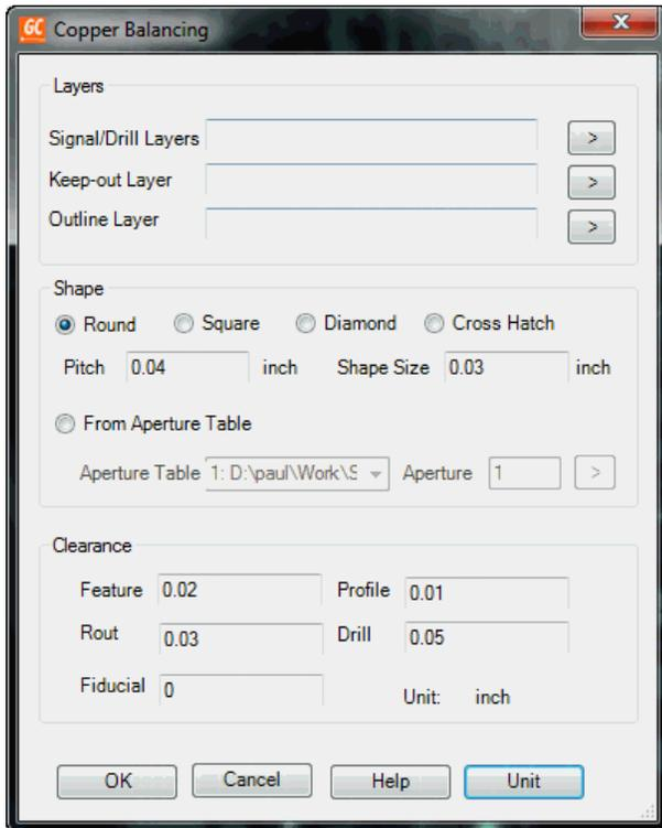
The function adds a user specified aperture, on a user specified pitch with various keep out distances around specific features. The function also allows a crosshatch pattern to be used. The additional pattern is added to a new data layer within each Signal physical layer to allow easy identification of the added data and allow additional user modification if necessary.
