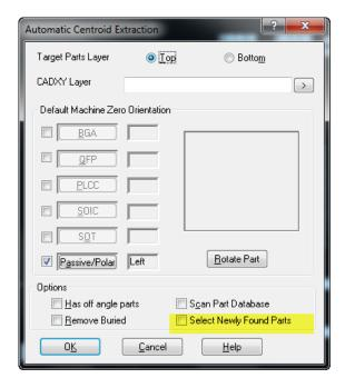
The idea is that by using the ACE function multiple times (for BGA,QFP,PLCC, then again just for SOIC etc.) the components found during each pass can be immediately verified in terms of rotation and centroid location.
