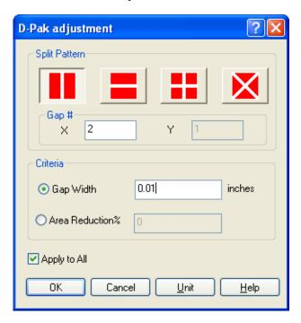
The function will be further enhanced with an area reduction option on rectangle pads.
